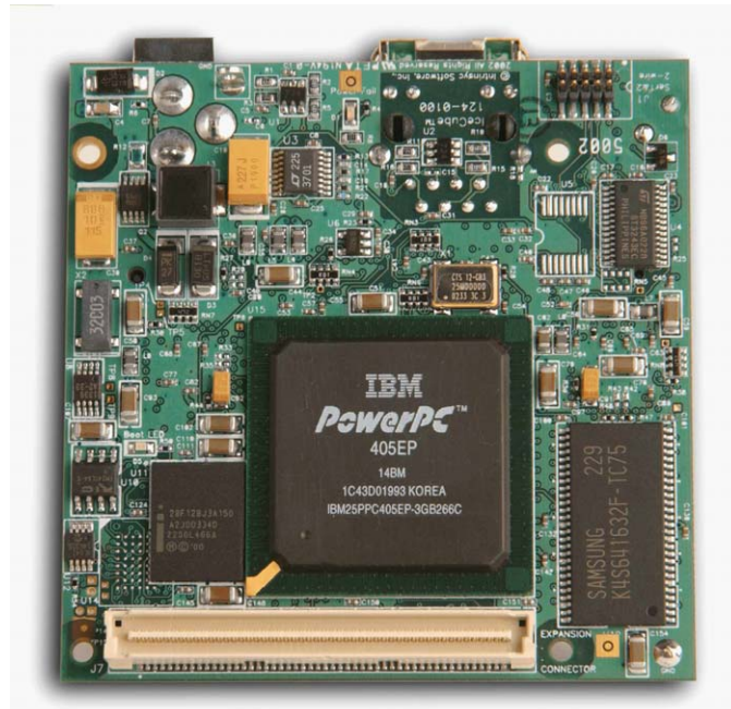
Intrinsyc's 405EP-based board, frontside
